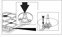
for burners with safety valve make sure that the regulation obtained is sufficient to maintain heating of the thermocouple. If it is not increase the minimum.
